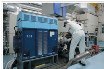
Oil pump test on engine dynamometer
